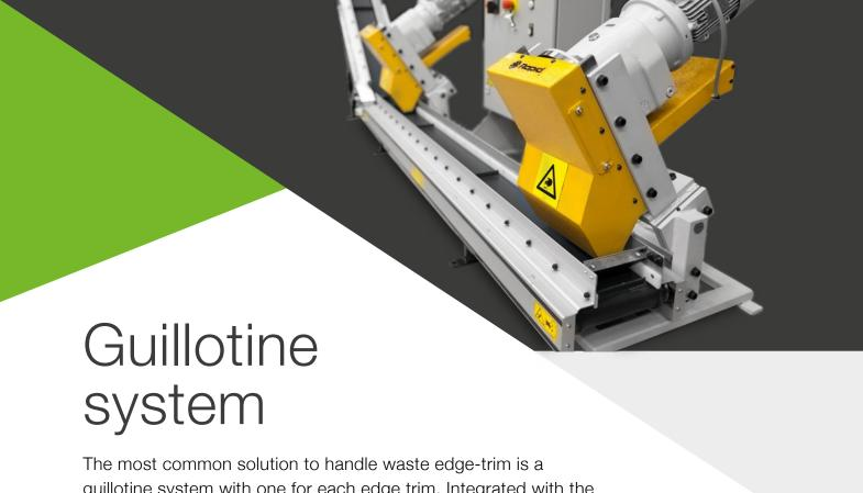
The most common solution to handle waste edge-trim is a guillotine system with one for each edge trim. Integrated with the extrusion line it continuously cuts the edge trims with the cut pieces falling onto a conveyor belt which is then fed to a granulator.
