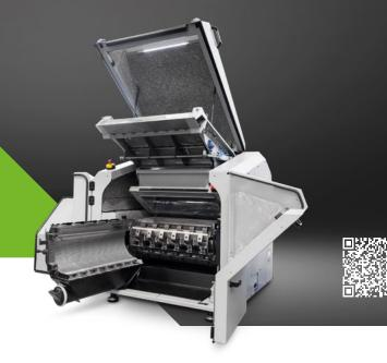
Rapid ThermoPRO for low noise granulation of skeletal waste.
